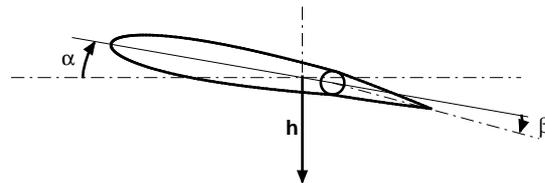
Figure 1: Airfoil pitching, plunging and rotation of the flap
