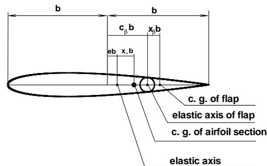
Figure 2: Typical airfoil section with three degrees of freedom.
