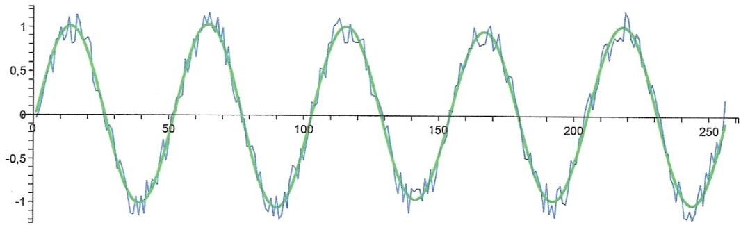
comparison of original and filtered signal
