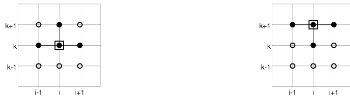
Figure 2: Grid nodes used for finite differences. Left: Four-point stencil for explicit method (it is centered at the node P_i^k ). Right: Four-point stencil for implicit method (it is centered at the node P_i^{k+1} ).
